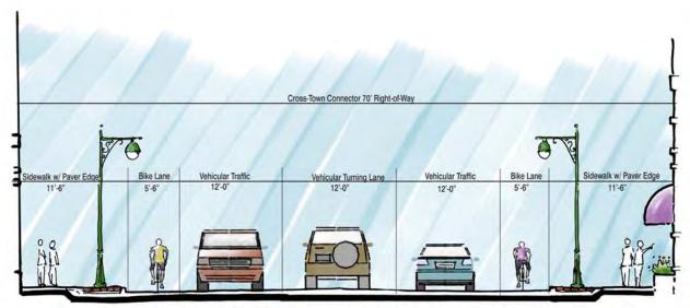
Proposed Cross-Town Connector Typical Cross-Section A
