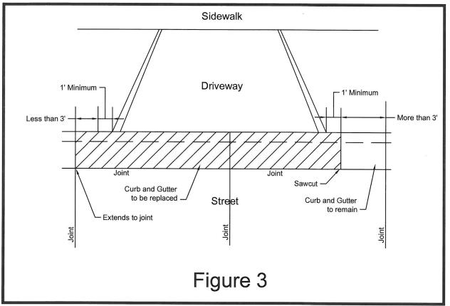
The replacement of a driveway requires the new driveway to conform to all specifications adopted by the City. Now driveways must abut the backside of the curb and gutter as shown in Figure 1. In the case where the existing driveway is cut into the street, as in Figure 2, the curb and gutter section must be replaced to conform to Figure 1. If the curb and gutter must be replaced, it shall be done so that not less than 3 feet remains to the next joint, as shown in Figure 3.
