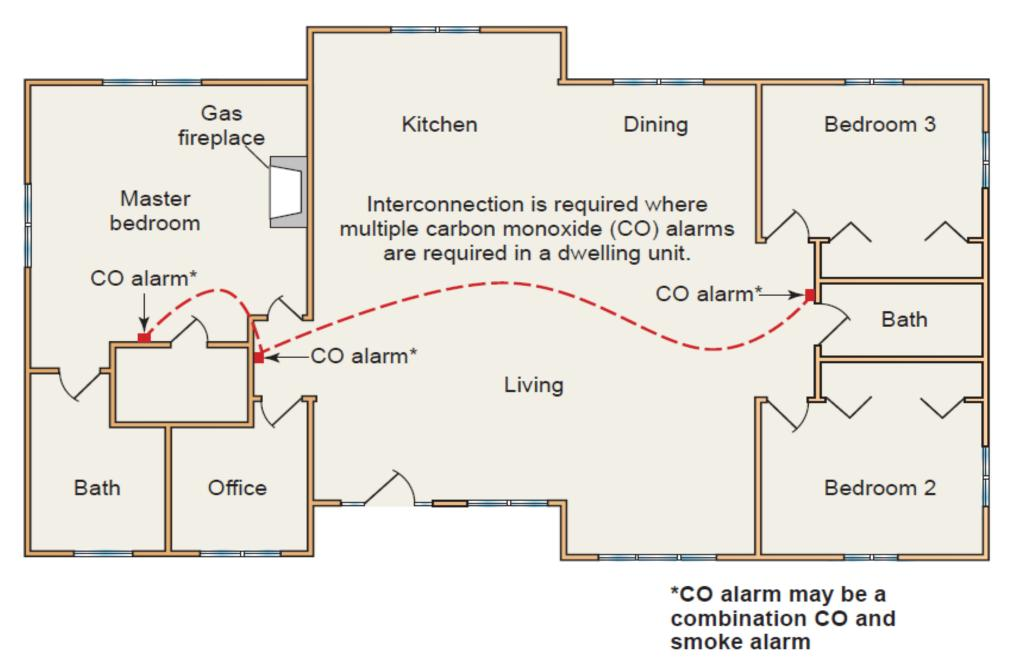
**FIGURE 10-3** Carbon monoxide (CO) alarm required in the immediate vicinity of each sleeping area and in bedrooms containing fuel-fired appliances
